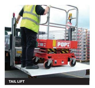
When using a forklift to lift the POP-UP PUSH 6 ECO, ensure the forks are sufficiently inserted into the forklift pockets in the base of the machine. Please see the location of the forklift pockets below. When using a tail lift to load or unload the POP-UP PUSH 6 ECO ensure that brakes are applied to both castors. Ensure that the capacity of the tail lift is sufficient to handle the POP-UP PUSH 6 ECO. Take care when manoeuvring the machine on the tail lift.
