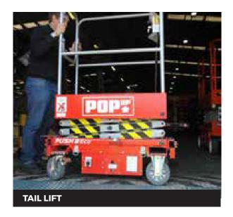
When using a forklift to lift the POP-UP PUSH 8 ECO, ensure the forks are sufficiently inserted into the forklift pockets in the base of the machine. Safety decals applied to the POP-UP PUSH 8 ECO show the location of the forklift pockets.
